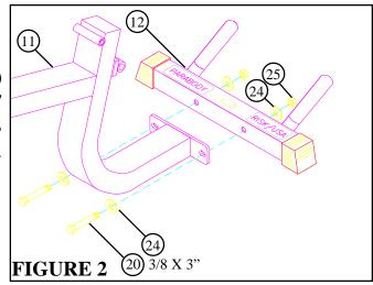
STEP 4: Securely assemble FRONT BASE SUP-PORT (1) to LEG FRAME (11) using two 3/8 X 3" BOLTS (20), four 3/8" FLAT WASHERS (24), and two 3/8" NYLOCK NUTS (25). See FIGURE 3.
